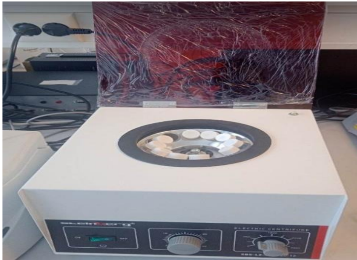
Figure 3.5: Sample inside centrifuge machine [Steinberg system SBS -LZ-4000 / 20 -12] for centrifugation process at USN lab.
