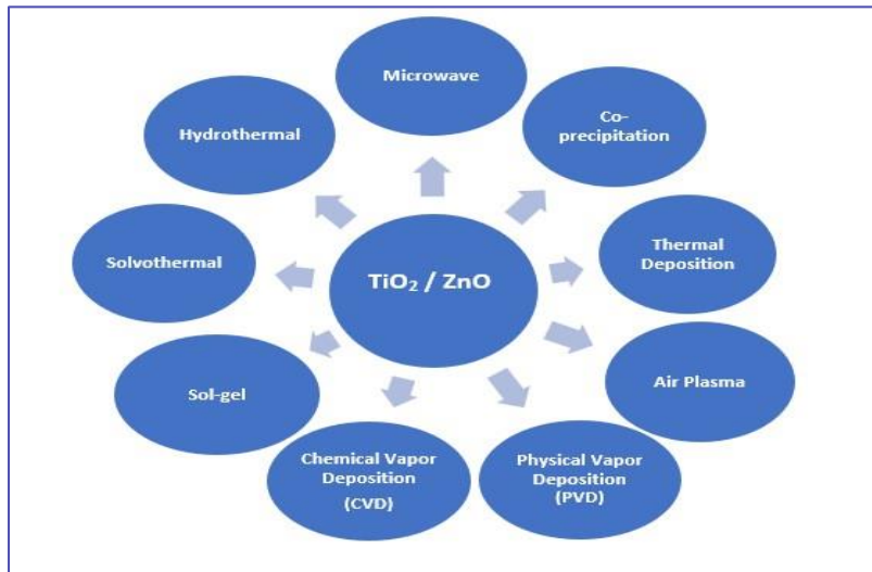
Figure 2.7: Common Synthetic method of TiO 2 /ZnO Nanostructure[43], [44].
