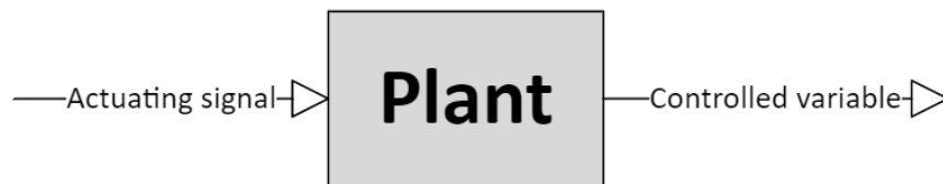
Figure 1, The plant is a system that we want to control its behaviors.
