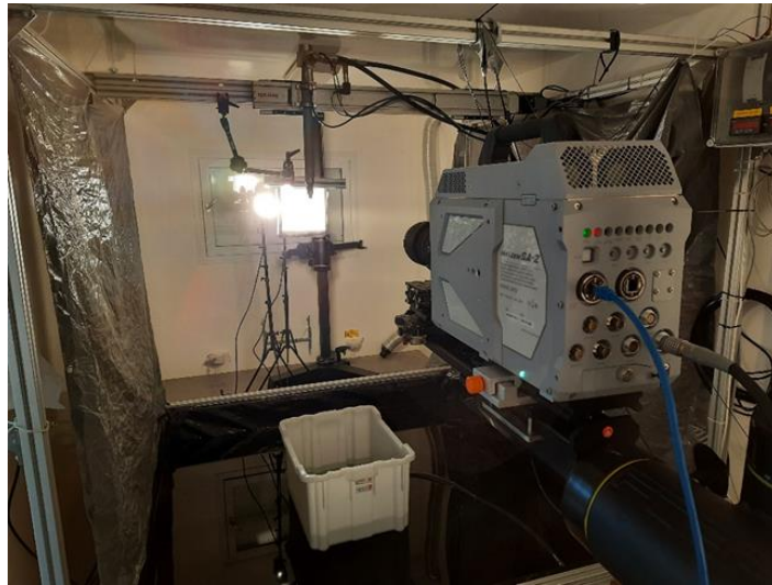
Figure 22. Backlight shadow imaging setup
