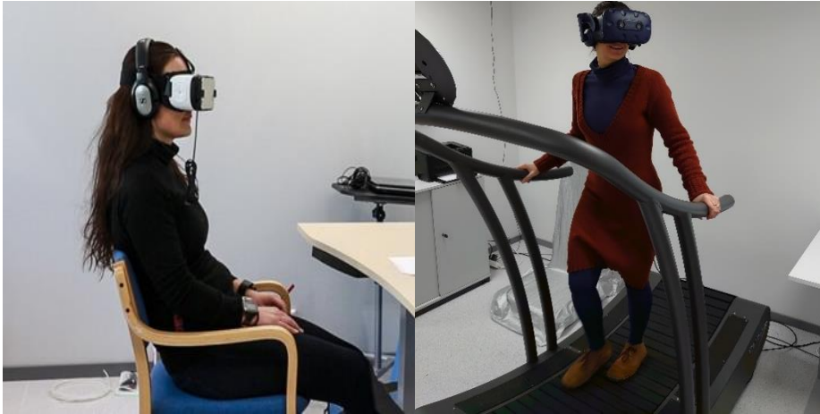
Figure 1: Examples of head-mounted displays (HMDs) in a sedentary exposure to virtual nature (left) and virtual green exercise (right).
