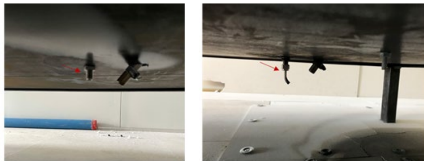
Figure 3.21: Nozzle configurations: left – 90° nozzle, right – 45° nozzle.
