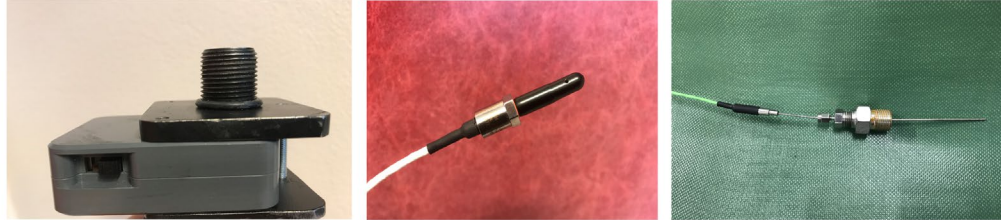
Figure 3.7: The sensor used during PPP experiments: XENSONR hydrogen sensors (left), Kulite pressure transducer (middle), and Thermocouple type K (right).
