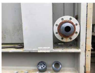
Fig. 2. The vent with variable area.
