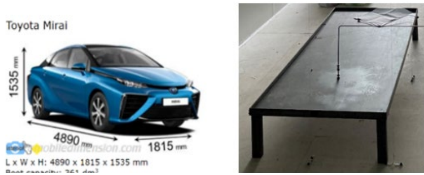
Figure 3.22: Picture of the table imitating the Toyota Mirai. Scaling factor 0.4.
