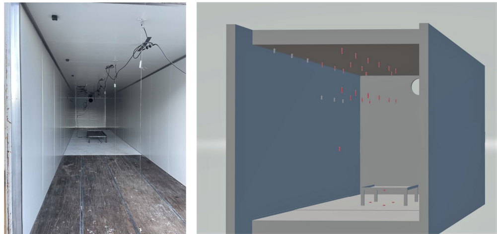
Figure 3.25: Hydrogen sensors' placement in the container. Red-CANbus sensors, grey-WIFI sensors.
