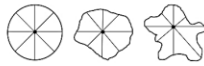
Figure 1. Shape factor measurement examples showing centroid and eight radii for each granule, with increasing shape factor left to right.
