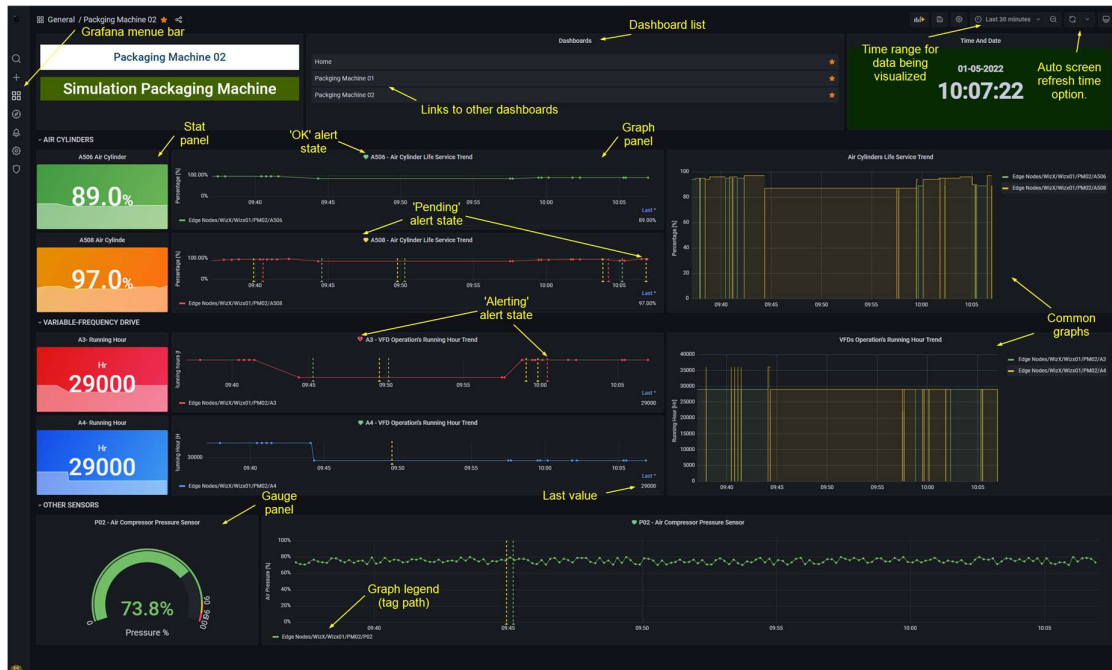
Figure 4.13: Screenshot of Packaging Machine 02 dashboard with yellow-colored annotations pointing to various parts of the dashboard.
