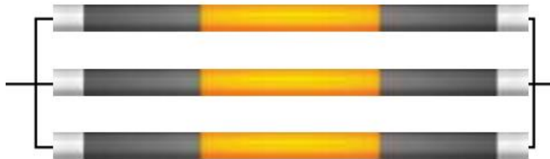
Figure 2-9: Case1, Heating elements in parallel connection [9]
