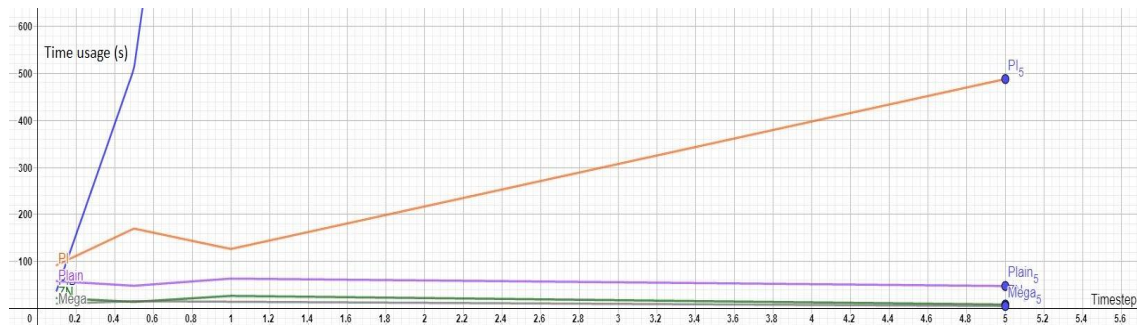
Figure 4-2: Test results of time usage (y-axis) from ZN, “pidstd(PI)”, “megatunerplain”, and “megatuner” using “rss”-created systems with varying timestep (x-axis)
