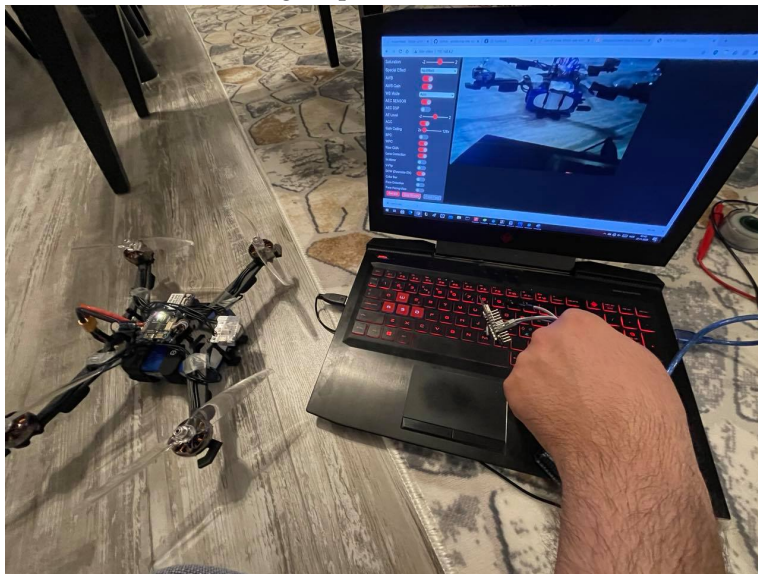
(B) Overall view of ESP32-CAM and the Drone
