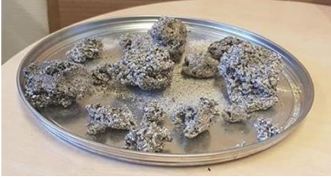
Figure 1. Agglomerates formed during gasification of biomass.
