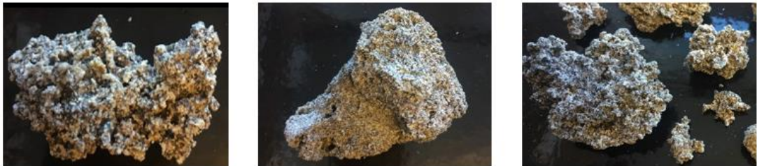
Figure 2-6. Agglomerated particles from biomass ash and silica sand particles formed during bubbling fluidized bed biomass gasification.
