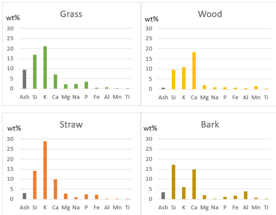
Figure 3-1. Ash content (black) and the compositions (wt % in ash) of the major ash forming elements for the grass, wood, straw and bark samples used in this study.
