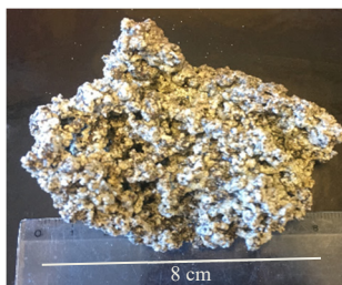
Figure 1: Agglomerates from biomass ash and silica sand particles.
