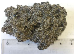
Figure 2. Agglomerate of biomass ash and silica sand particles, formed in a bubbling fluidized bed gasifier.
