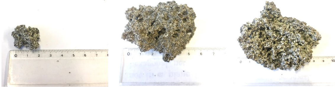
Figure 6. Agglomerates from fluidized bed gasification of biomass.
