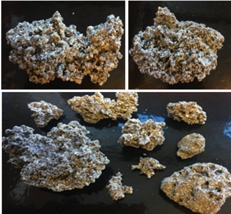
Figure 2: Agglomeration of silica sand particles.
