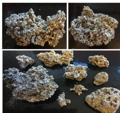
Figure 2. Agglomerates from silica sand particles.
