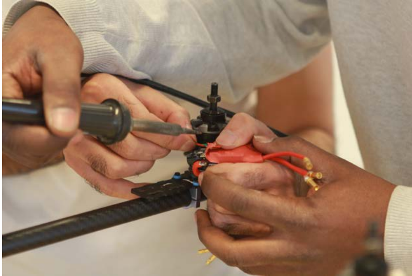
Figure 5 soldering and attaching the ESC and motor to the arms
