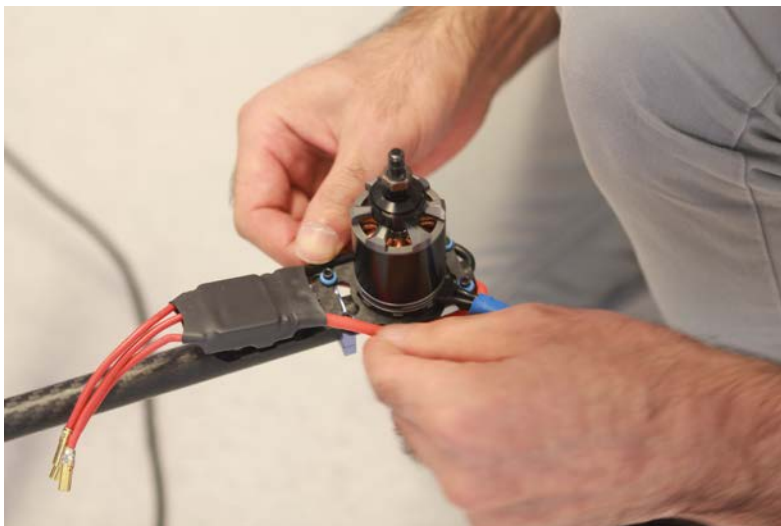
Figure 6 Shirked tube around the ESC
