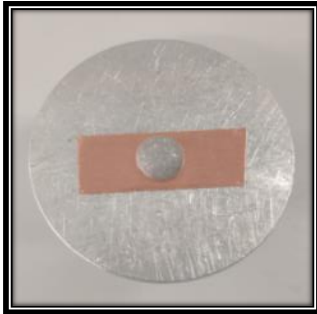
Figure 2.8: 50-50% of phosphor and glass ratio after sintering process
