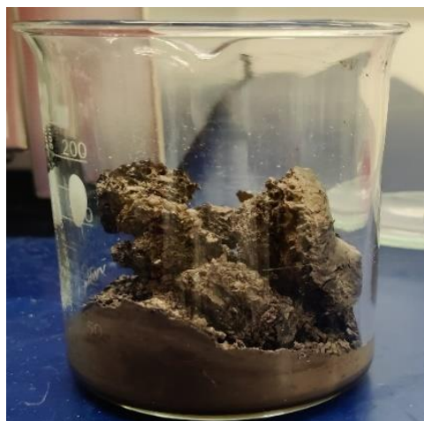
Figure 2-4: Black substance formed after pre-calcination of yellow gel
