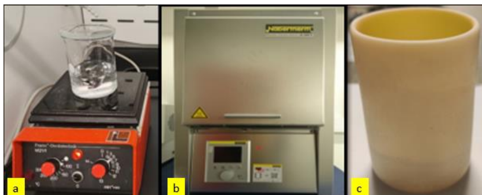
Figure 2-2: (a) Hot plate oven with magnetic stirrer (b) High Temperature furnace (c) Crucible for calcination purpose
