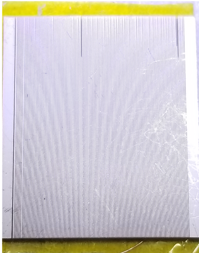
Figure A.4: Diced PZ-27 with air kerf and Kapton tape on the bottom. Feedspeed = 1 mm/s. Shower rate = 0.75 L/mm.
