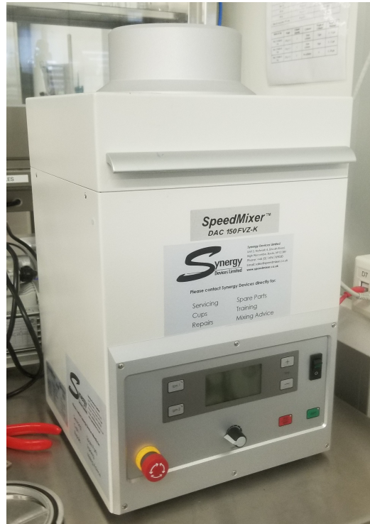
Figure A.6: Mixing of epoxy with Speed Mixer DAC 150 FVZ-K
