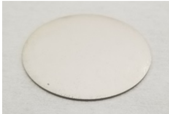
Figure A.1: Bulk PZ-27 disk with diameter of 3 cm supplied from manufacturer FerroPerm A/S
