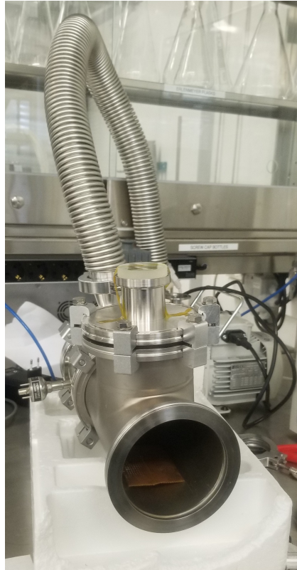
Figure A.7: Degassing setup for epoxy.
