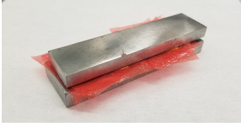
Figure A.9: Filled samples sandwiched by insulating tapes and metal brick to avoid bending of the sample.
