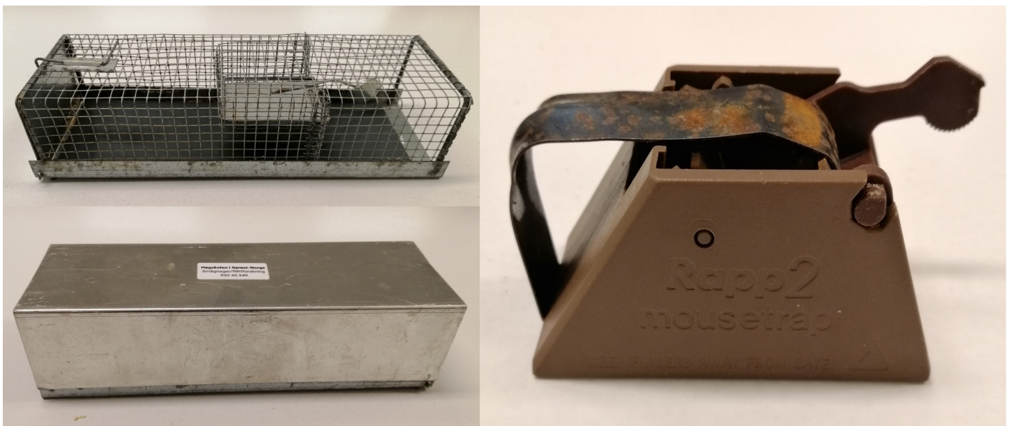
Fig 1. The two trap types used in the study. (A) Uggulan special Nr 2 live trap (top), covered with an Uggulan special long roof metal cover (bottom). (B) Rapp2 lethal mousetrap.
