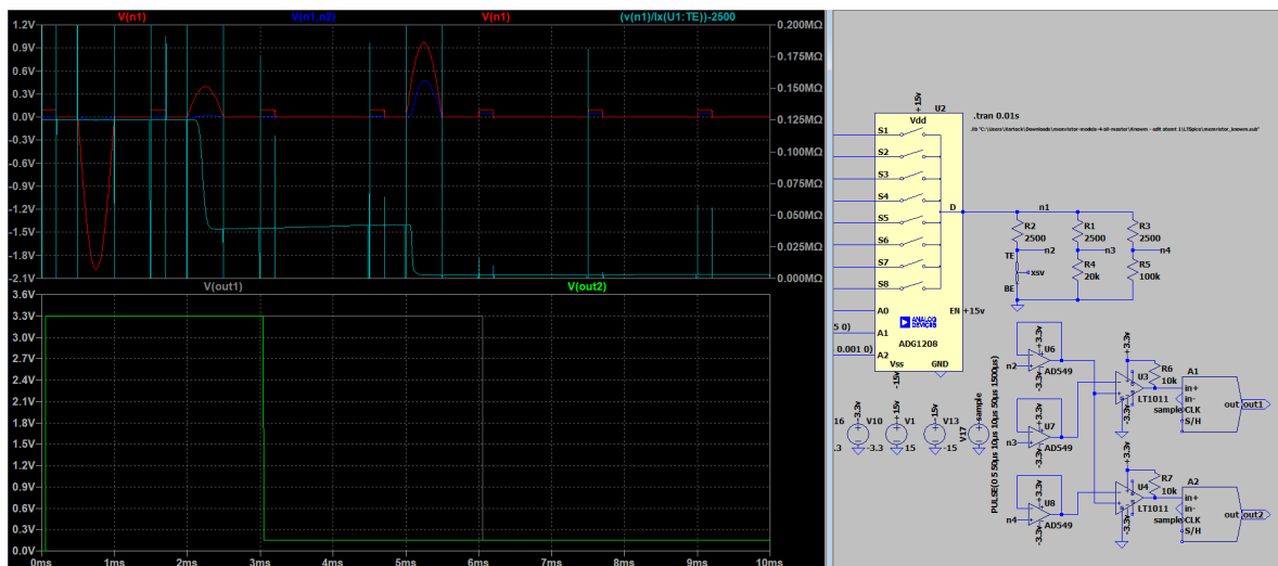
Figure B.63: Here I decided to use state/hold elements on the output insted of before the comparison because the levels before the comparison are more crucial that they are correct and tle outputs do not need to be as exact, this seem to work well and the states save between read pulses well. the read circuit seems to funtion correctly now.
