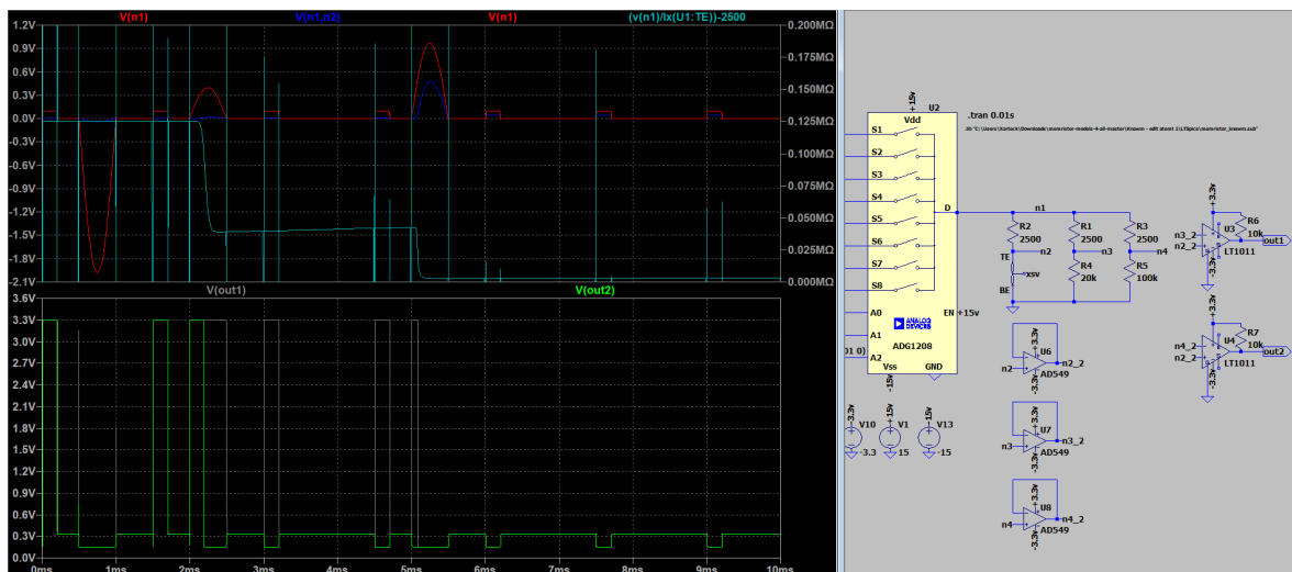
Figure B.61: In this iteration I have fixed the comperators and graph thair output, there is no hold or selection on when to compare in this iteration.
