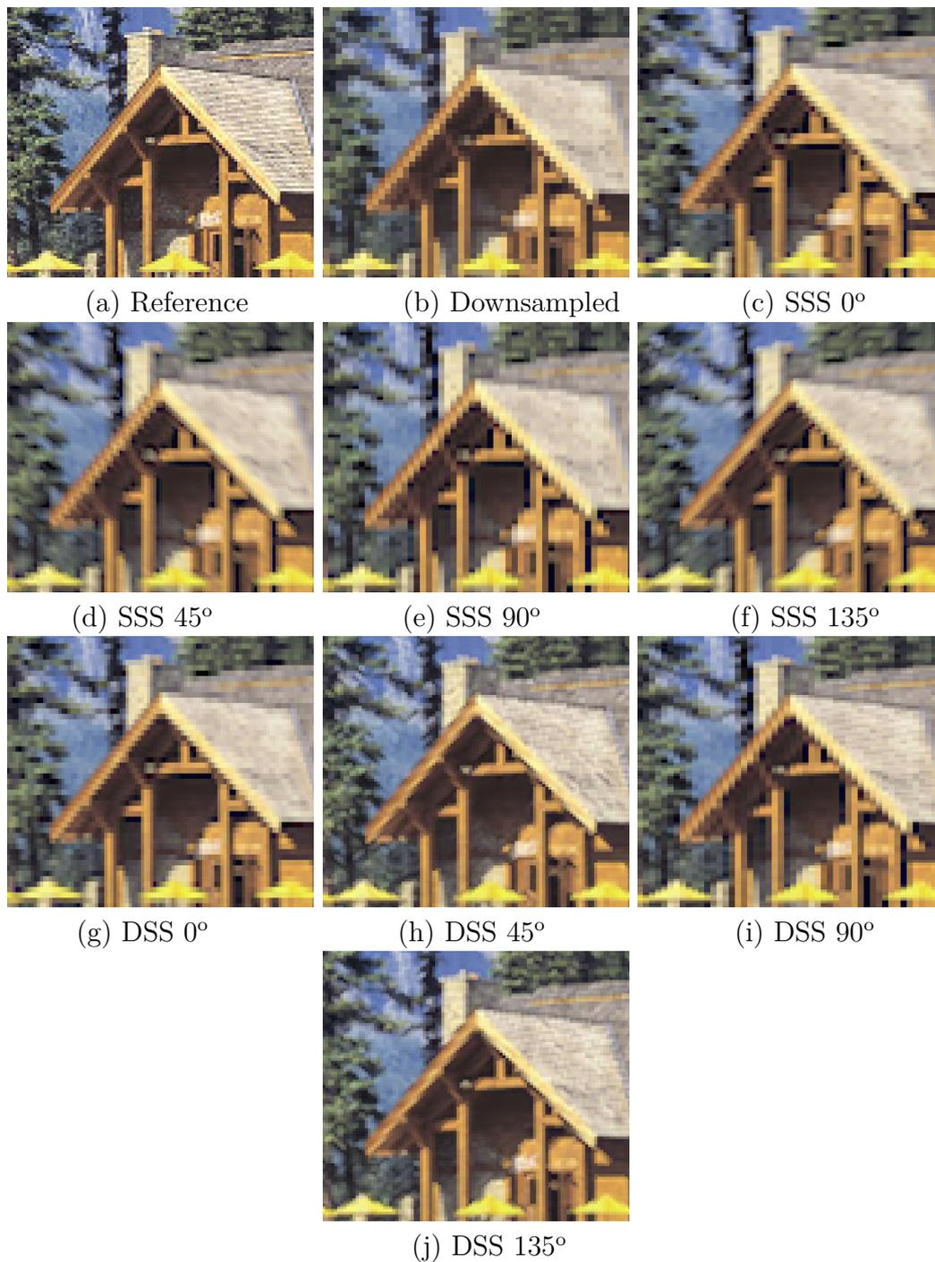
Figure 4.3: Cutout of a forest cabin image. a) reference image, b) downsampled to SLM resolution c) SSS 0°, d) SSS 45°, e) SSS 90°, f) SSS 135°, g) DSS 0°, h) DSS 45°, i) DSS 90°, j) DSS 135°. SSS notes the Single Subframe Shifting while DSS notes the Different Subframe Shifting. Notice the image artefacts appearing in different directions according to the direction of the shift.
