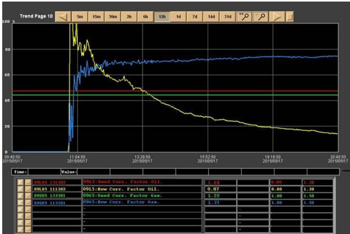
Figure 26 - Not acceptable k-factor development through traditional calibration on the metering system on Alvheim
