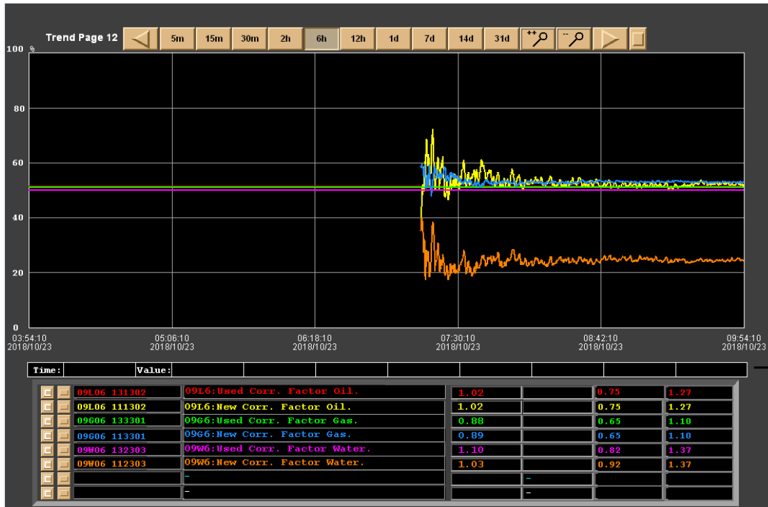
Figure 27 – Acceptable k-factor development through traditional calibration on the metering system on Alvheim
