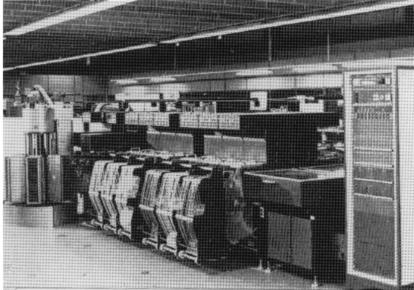
Fig. 7.36: Philips large hardware controlled pick-and-place machine.
