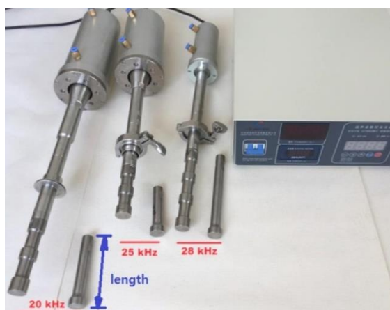
Figure 11. The sonotrodes used depicted. Note the different length of the sonotrodes of 20, 25, 28 kHz (the 25 kHz being the shortest)
