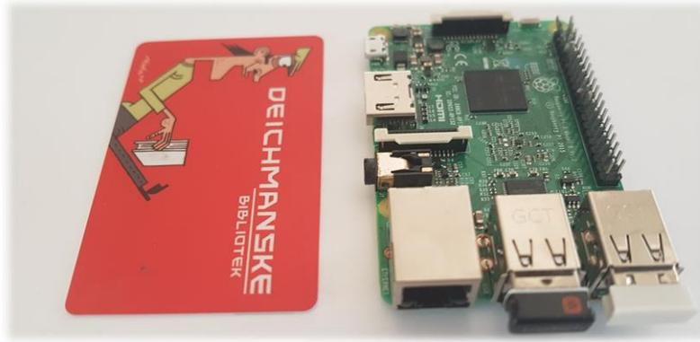
Figure 1.1 - The Raspberry Pi 3 Model B, with a size similar to a credit card.
