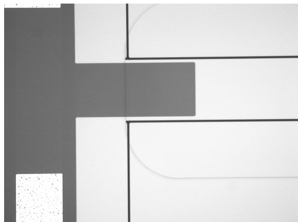
Fig. 16. The base of the beam with cut through areas seen as black lines. Nominal line width 3 microns. The rounded corners indicate the position transition from thick to thin membrane.
