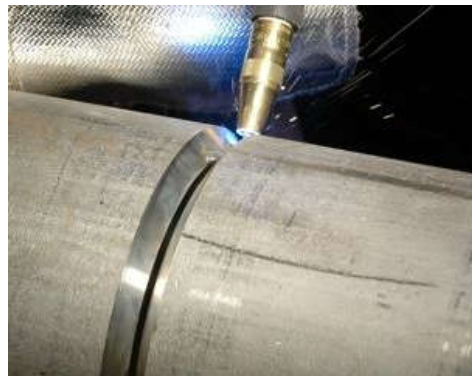
Pictures showing flanged and buttwelded pipe (Explore the world of piping, 2017).
