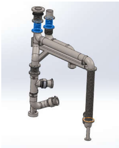
Picture shows the two swivel joints in blue (Designed in SolidWorks by bachelor group).
