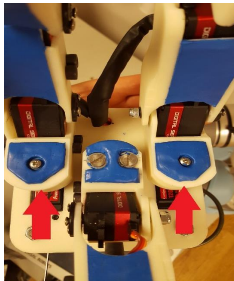
Figure 19: Attaching finger to the servo on top cabinet panel
