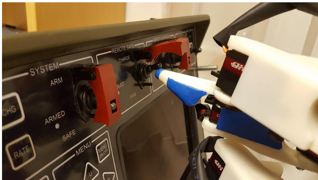
Figur 41: Fingertupp vipper indre bryter.
